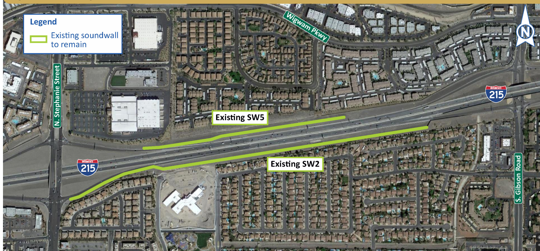
Figure 3.7 Existing Soundwalls in Areas 2 and 5
